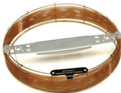
A special tab clearly distinguishes the EZ-Guard guard column section from the analytical column
