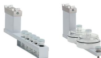
The Fast Wash Module is preferred when **low carry-over** is required. It also cleans syringes incl. the outside of the needle (gauge 19 – 26) with 2 different solvents.
