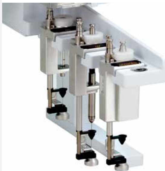
Park Station with Liquid, SPME and Headspace tools
